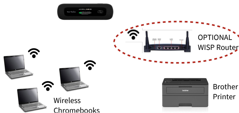
Figure 3: Network Options 4 and 5: Tax-Aide private sub-network using Hotspot with or without router.
